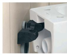
The use of a specially developed connector with the same length as the distance between the threaded rods of the wall carrier eliminates the need for further adjustment. The SupraFix 2.0 carrier supports the toilet while installation is completed.
